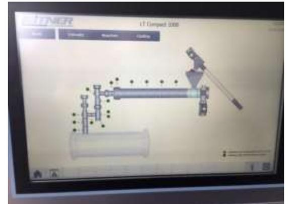
Fig. 8 Control screen showing component process monitoring
