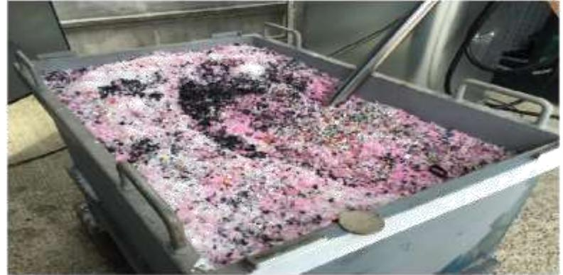
Fig. 2 The plastic pellet bin with attached vacuum hose
