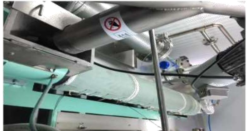
Fig. 3 The plastic enters the depolymeriser via an auger
